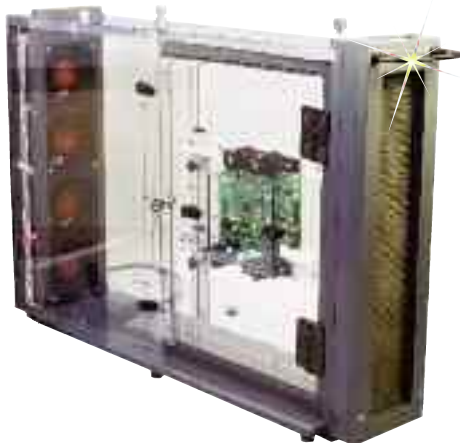
Figure 3 –Benchtop Thermal Evaluation Wind Tunnel (Omega Engineering, Inc.)
