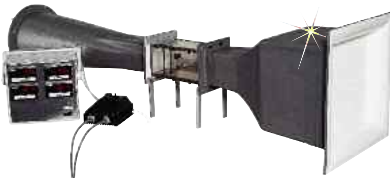
Figure 1 –Laboratory-Grade benchtop wind tunnel shown with control panel (Omega Engineering, Inc.)
